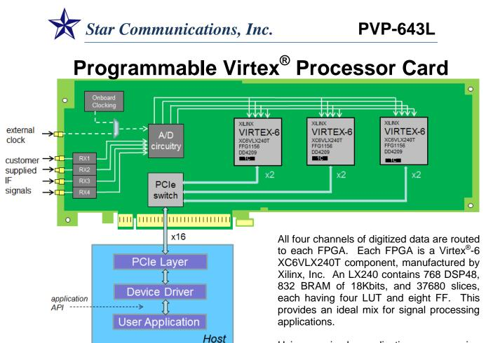
The PVP-643L card combines a multichannel digital receiver with FPGA-based signal processing elements, on a standard PCI Express<sup>®</sup> (PCIe<sup>®</sup>) card. When installed in a customer's host system, such as a rack-mount server or other PCIe host, a PVP-643L provides a complete IF-to-DMA path for receiving wireless signals, processing them in an FPGA, and sending results to host CPU(s) via PCI Express.
